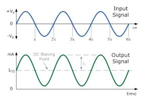
A Class-A amplifier configuration uses the same switching transistor for both halves of the output waveform and due to its central biasing arrangement, the output transistor always has a constant DC biasing current, ( $I_{CQ}$ ) flowing through it, even if there is no input signal present. In other words the output transistors never turns "OFF" and is in a permenant state of idle. hence it requires a heat sink as DC is lost as heat.
